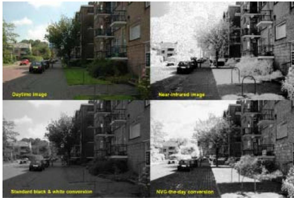
Fig. 16 NVG-the-day color transformation. While a standard black-and-white conversion looks very different from the near-IR (NIR) image, the NVG-the-day result closely resembles the NIR image.
