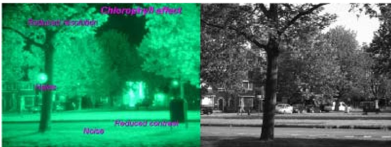
Fig. 15 The differences between (right) black-andwhite daytime images and (left) night-vision goggle (NVG) performance.
