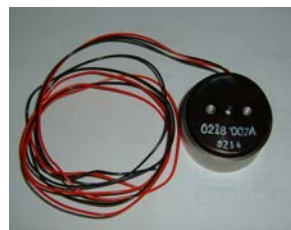
Fig.4a. The voice coil.
