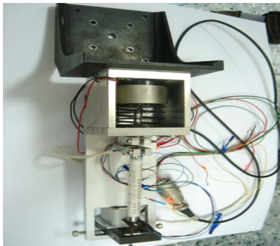
Fig.9 the integration module of voice coil, LVT & LVDT.
