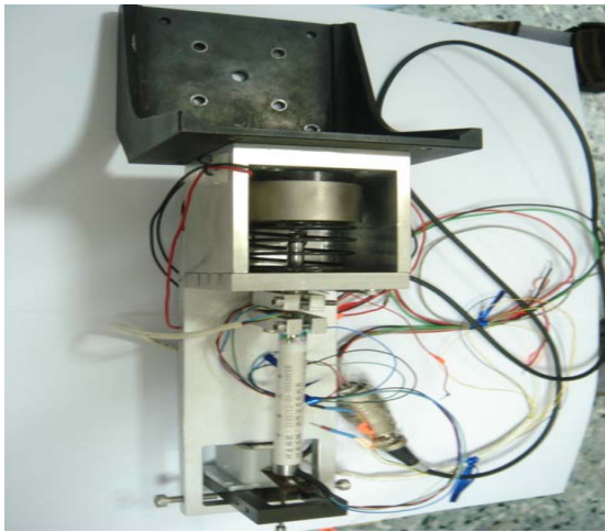
Fig. 5d. Integration of voice coil, LVT & LVDT.
