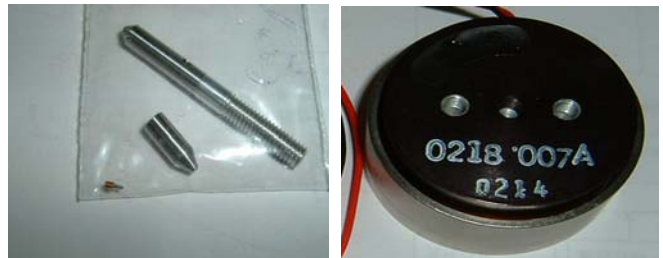
Fig.2 the LVT is to detect the vertical velocity of the stylus probe.
