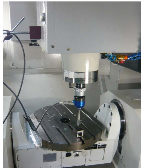
Figure 6. R-test measuring in machine tools
