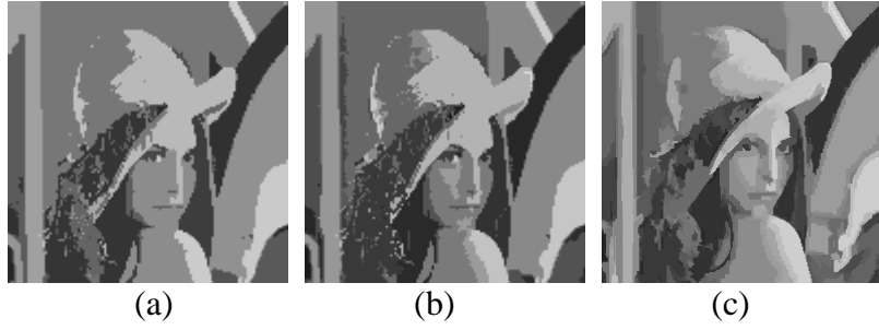
Fig. 2. The Lena image is partitioned into 300 regions using (a) RSST, (b) FRSST, and (c) MFRSST algorithms.
