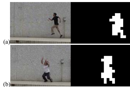
Fig. 6 Images on the left side show the moving human with different actions and images on the right side illustrate the segmented regions.
